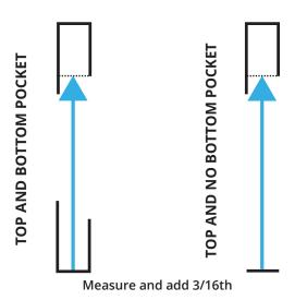
Measure from where the screen will rest on the sill to the opening of the top screen track/pocket (shortest leg),
